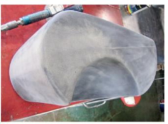
Sand the seams flush with the plastic tank sides, being careful to keep the block or DA sander flat. You will need several discs or pieces of sandpaper for this as it will get dull or clog with plastic.
