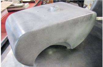
Wet sand with 400 grit wet/dry sandpaper and a semi hard sanding block or foam pad for best paint prep results.
